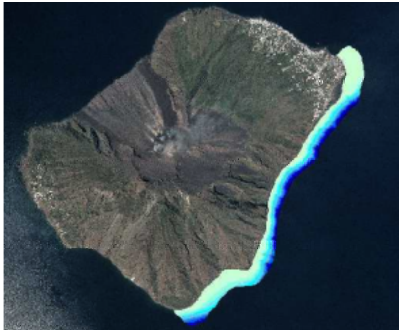
Fig.2: Resulting DTM from bathymetric surveys performed within the 2 nd year
